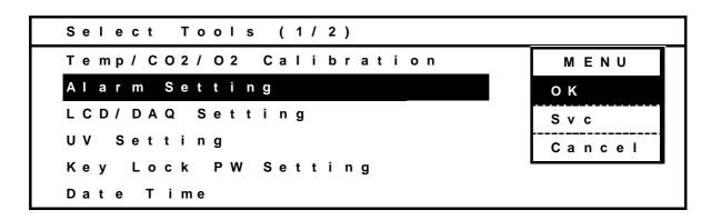
**3.** The Alarm Setting Display will appear. The temperature alarm,  $CO_2$  alarm,  $O_2$  alarm, alarm delay, ring back time, and door delay can be set on this display. The alarm buzzer can be silenced by pressing the BUZZER Key. The buzzer will sound again after the specified ring back time if the condition that caused the alarm continues. The ring back time can be set.
